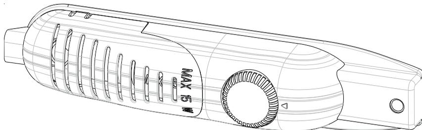
Thermostat automatically regulates the inside temperature of the refrigerator compartment and freezer compartment. By rotating the knob from position 1. to 5., colder temperatures can be obtained.
