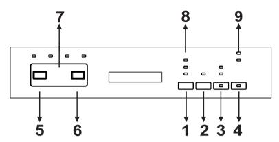
By pressing On/Off button(4), energise the machine. On/Off lamp lights as long as the machine is on.
