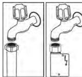
**NOTE:** Aquastop water spout is used in some models. In case of using Aquastop, a dangerous tension exists. Do not cut Aquastop water spout. Do not let it get folded or twisted.
