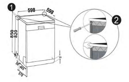
Warning: The stand part which we will settle our machine under it by removing its worktop has to be stable in such a way not to allow balance disorder.
